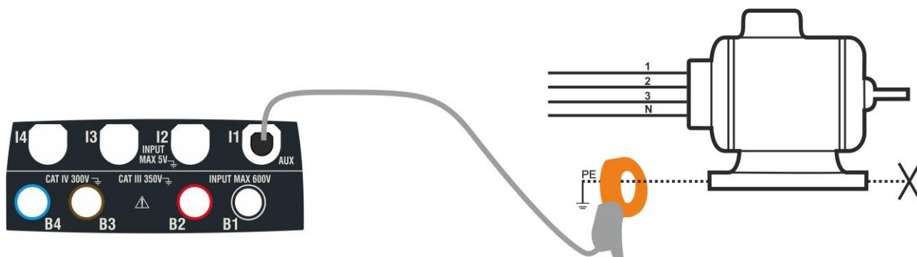
Fig. 7: Direct measurement of leakage current in three-phase systems
